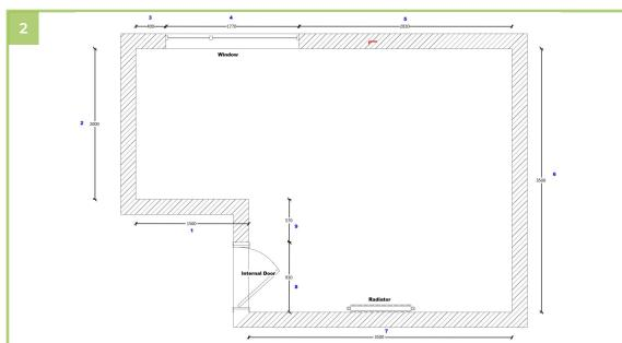
Start in a corner and measure each individual section of wall. Eg. Between corner of room and window, window and door etc. Continue until you've completed the room. NB: If possible please use metric measurements (mm or cm)
